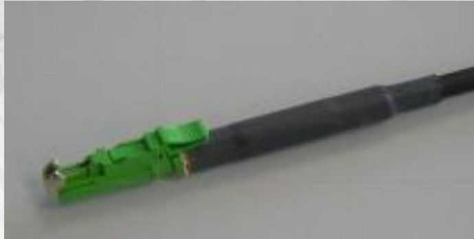
Optical fibre connector mounted on the sensor cable
